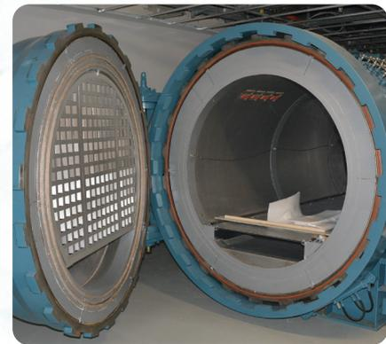
**Autoclaves** are essentially heated pressure vessels usually equipped with vacuum systems into which the bagged lay-up on the mould is taken for the cure cycle. This advanced composite process produces denser, void-free mouldings due to elevated heat and pressure used for curing. It is widely used in the aerospace industry to fabricate high strength/weight ratio parts from pre-impregnated high strength fibers for aircraft, spacecraft and missiles.
